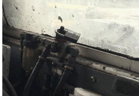
Methane monitor system bypass lock on a vehicle.
