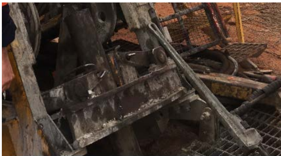
Photo 1: Foot clamp table C-section before guarding.
