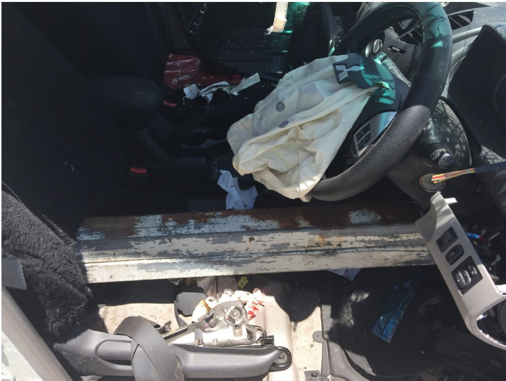
Photograph 2: Section of steel gate and driver's cabin of private vehicle.
