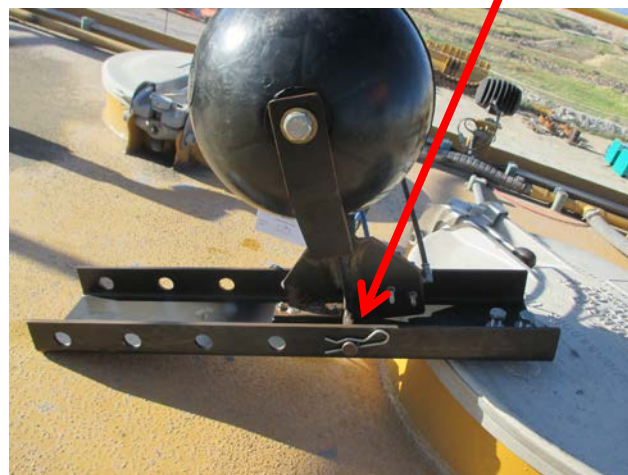
Figure 2: View of burnt breather vent and the setting of the diesel ball float valve in the support bracket.
