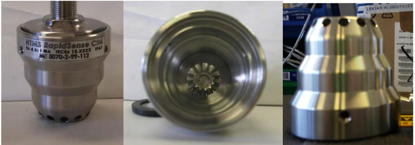
The modified housing (shown in figure 2 below) has six outside gas entry holes and a centre hole with six gas entry holes to the interior. Note also that the modified housing is taller.
