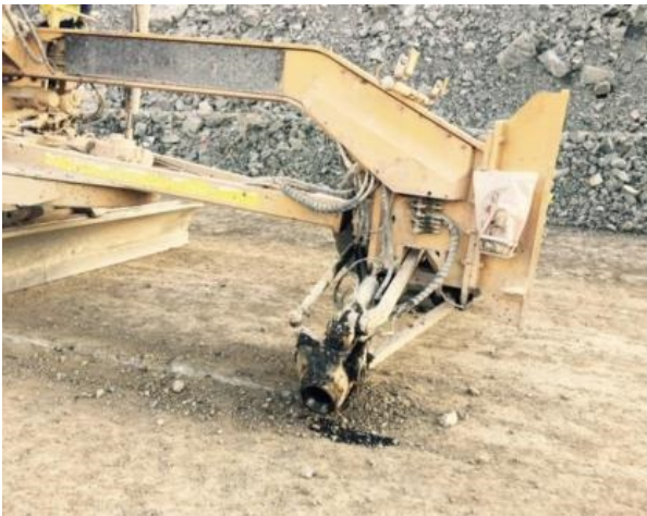
Example of a steering wheel failure and a driving wheel failure.
