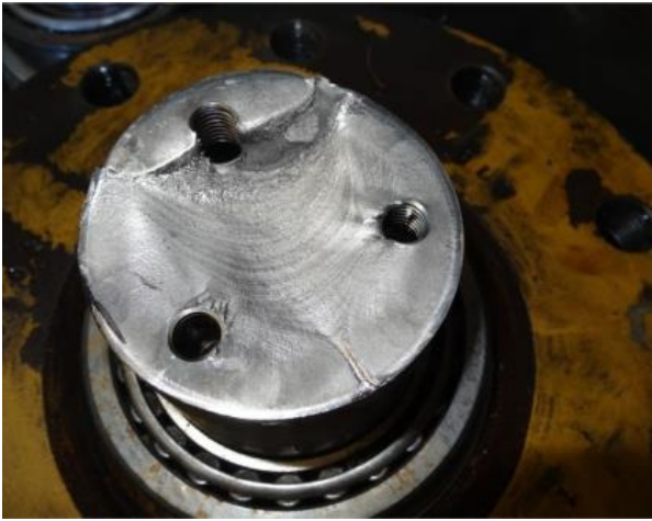
Progressive fatigue failure on a steering stub axle and a steering stub axle failure due to suspected shock load.
