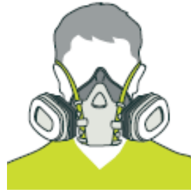
FIGURE 1: Re-usable half-face respirator (cartridge)
