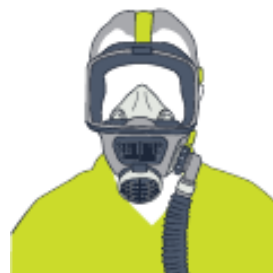
FIGURE 3: Full-face powered respirator (cartridge)
