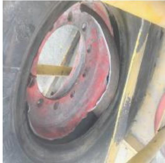
The leading hand was walking away from the tyre when he heard a large bang. The tube had failed and a high-pressure air blast hit the worker.
