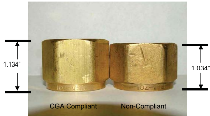
Figure 1 Measured length (shown upright) on CGA compliant and non-compliant high pressure oxygen fitting (nut)
