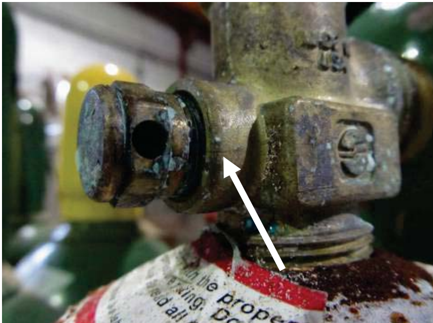
Figure 2 – View of cracked cylinder valve. Arrow points to crack.
