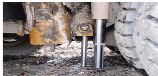
Hoist Cylinder Failure
