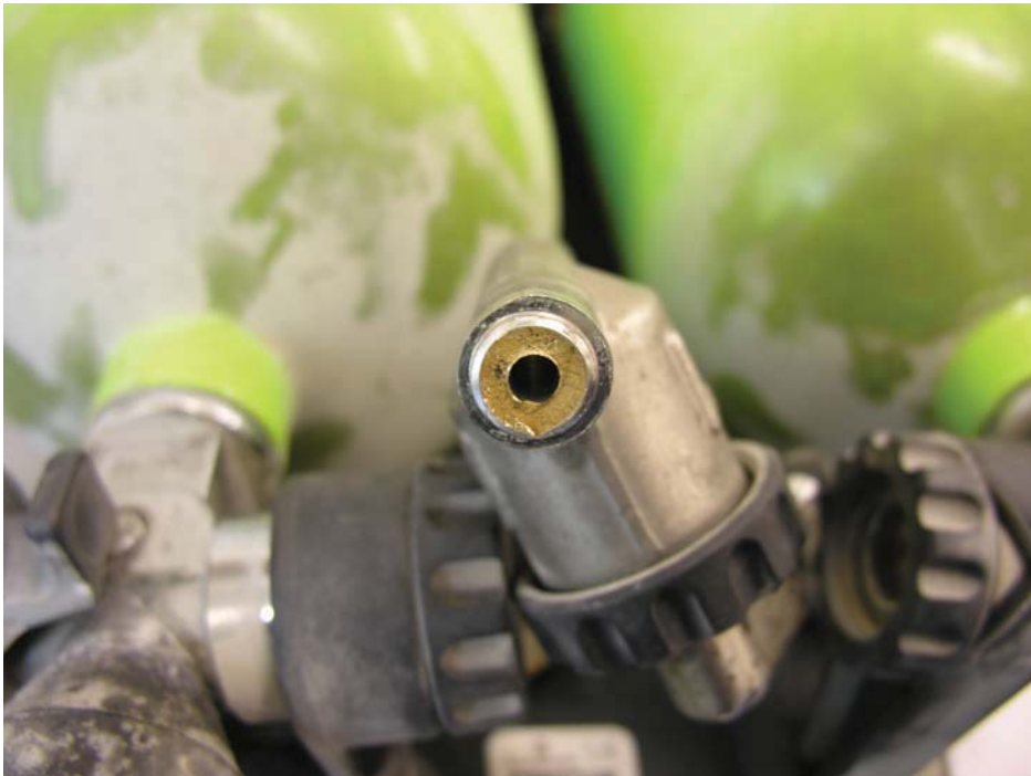
CABA unit showing broken connection
