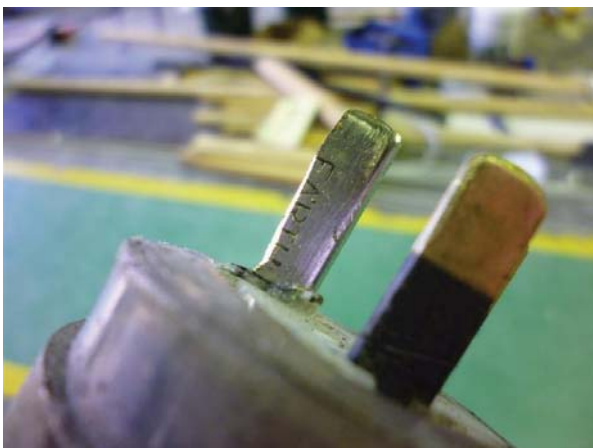
Example of a 3 pin plug with the earth pin filed down to enable use in a 10A socket outlet.
