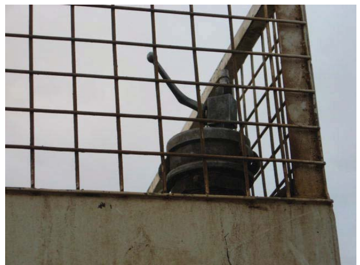
3" Cam lock fitting used to inject compressed air into the refuelling pod
