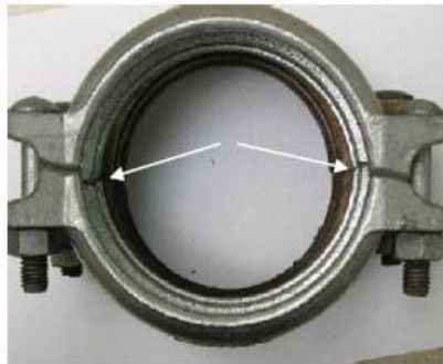
Image of SC77 coupling showing areas with reduced overlap due to the oval design of the fitting
