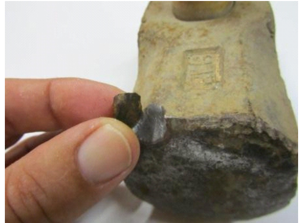
Hardened steel sledgehammer with steel shard
