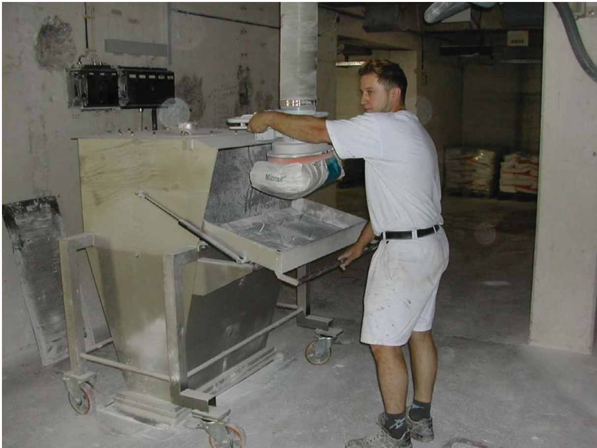
Fig. 3: Bag emptying station
