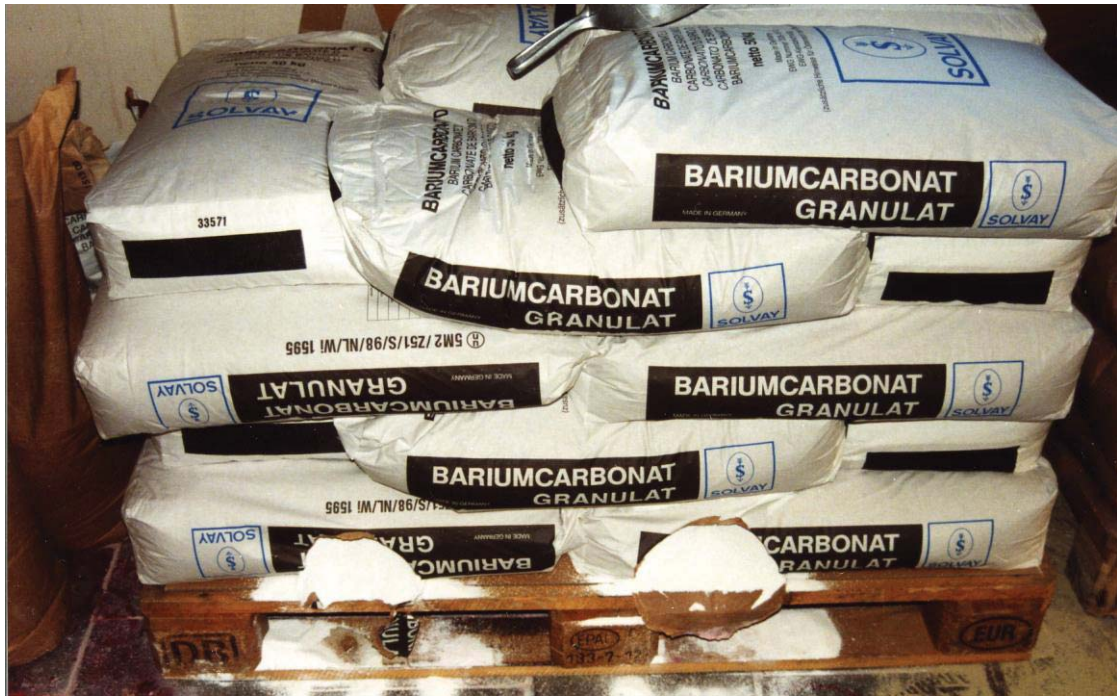
Fig. 2: Barium carbonate sacks damaged by plant-internal traffic; the raw material is provided as granulate
