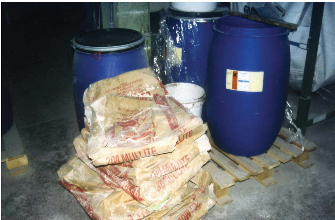
Fig. 4: Dust source as a result of the storage of empty paper bags
