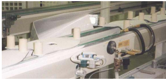
Fig. 2: Combined blowing/suction device for cleaning kiln furniture
