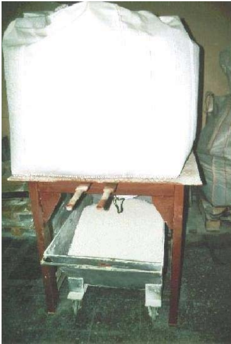
Fig. 2: Low-dust workplace as a result of using granulate
