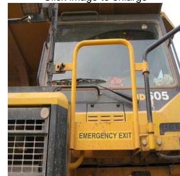
Close up of gate at top of emergency exit ladder
