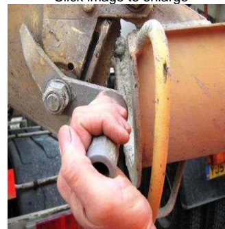
Shute with Missing Bolt
