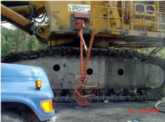
Figure 1: Failure of lift from improper welding
