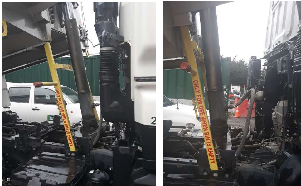
Photos: Left – Truck deck elevated above the deck restraint frame; Right – Properly deployed deck restraint (bin lowered onto the restraint frame);
