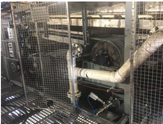
Figure 4 – Proximity of filter to the open guard door
