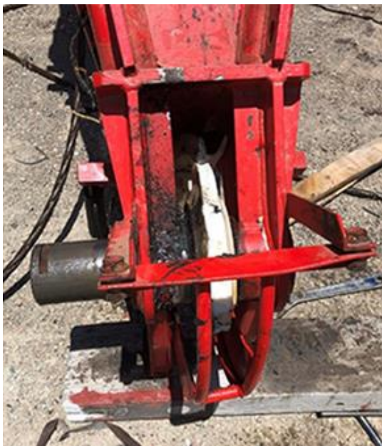
Photograph 2: Failed rooster sheave (180-tonne crane)
