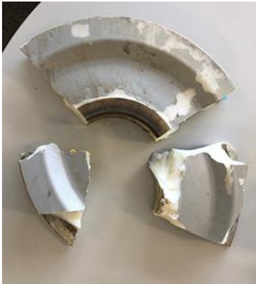
Photograph 1: Failed sheave segments (130-tonne crane)
