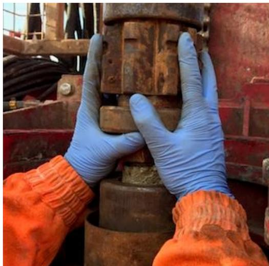
**Photo 2 – use of lay key and wire rope to release latches.**
