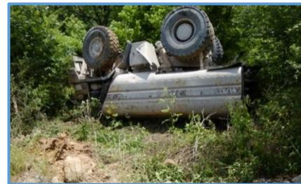
*This water truck encountered a soft road shoulder, overturned and rolled down an embankment, The operator was wearing a seat belt and was uninjured.*
