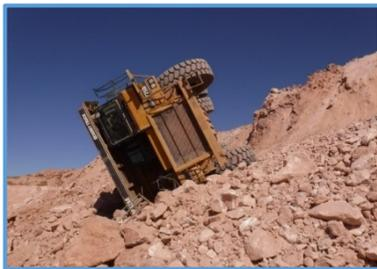
*This haul truck was dumping at the edge of an over-steepened stockpile. He was wearing a seat belt and suffered only minor injuries.*
