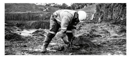
The sequencing of blastholes permits the controlled release of explosive energy in a manner that provides the required level of confinement and burden relief to achieve the desired fragmentation and blast movement, while minimising the risk of undesired outcomes such as flyrock, overpressure, vibration, noise, misfires and poor fragmentation.
