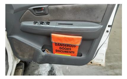
Bulk explosives delivery records by truck and shift should be kept, that allow reconciliation of actual and design densities and quantities, of explosive products used, and identification of which holes were loaded by which truck. The manifests carried on any vehicles carrying initiating explosives should enable reconciliation of explosives stock.
