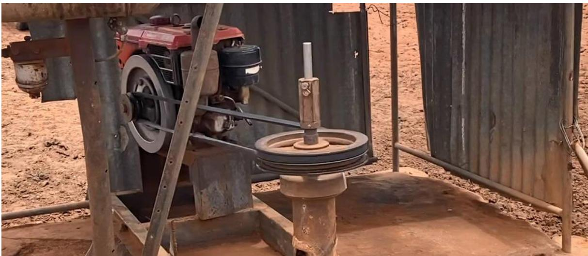
**Image 1:** The pump's moving pulleys and belt unguarded, are a hazard for nearby workers. (Source: NT Police)
