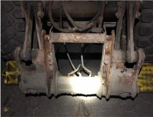
*Figure 1. LHS locking pin partially extended*
