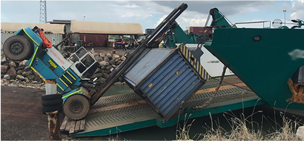
**Incident 2:** Travelling with a raised load weighing above the forklifts rated capacity increases the risk of tipping.
