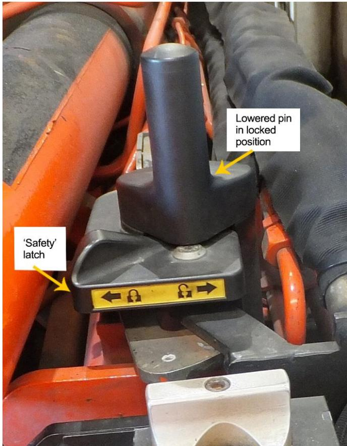
**Photograph 2:** Main pin, secondary steel latch and plastic latch in locked position with stabiliser stowed.
