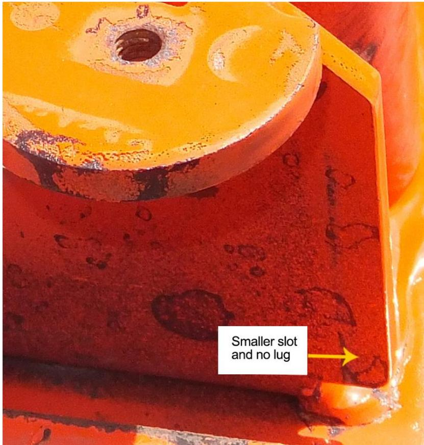
**Photograph 4:** Older design showing similar location to Photograph 3 (parts removed for clarity) – spring cannot be fitted without significant modification.
