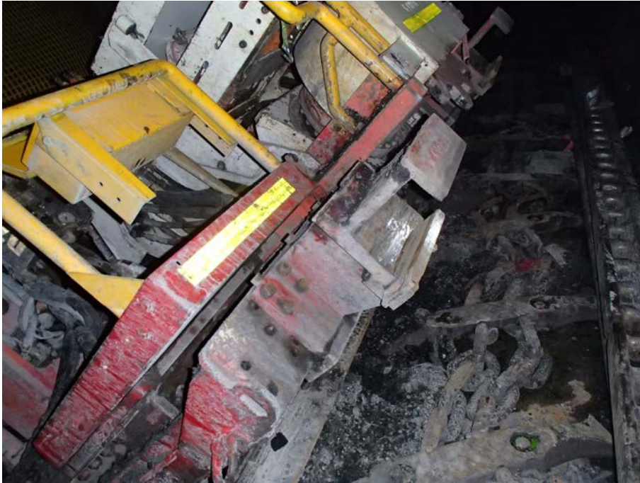
Figure 1 Rapid face bolter tipped 45° towards the face
