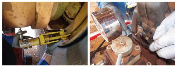
Re-enactments showing approximate hand grip on the bead breaker and position of power cable under the toggle switch
