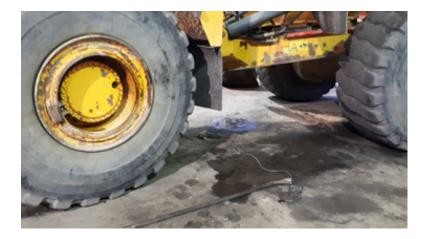
A crowbar was left leaning upright against a light vehicle in the workshop when workers left for smoko. The crowbar fell severing an electrical extension cable on the floor of the workshop.
