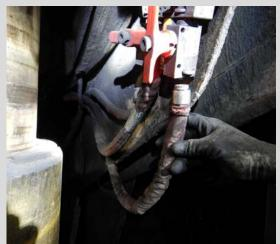
An escape of pressurised fluid in the workplace represents a failure of a risk control to a major hazard (pressurised fluids) that may cause serious or fatal injury. Mine operators are reminded that effective isolation, correct use and understanding of out of service tags procedures and energy dissipation are critical risk controls when working on high pressure fluid systems.
