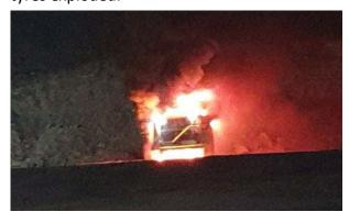
The investigation is ongoing, however good maintenance practices are essential to preventing fires on mobile plant. Heat shields and lagging designed to prevent combustible materials from contacting hot surfaces must be regularly inspected and maintained. Maintenance practices should also include securing loose combustible items to prevent contact with hot surfaces.
