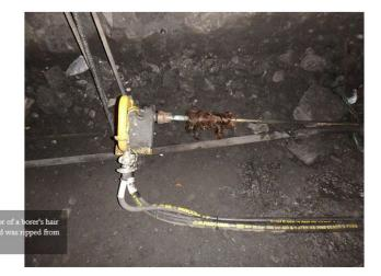
In a mine incident, this past week an operator's hair was ripped out following entanglement with a handheld borer. The incident highlights the risks of entanglement of clothing and body parts when working with machinery.
