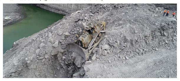
Figure 2 Dozer rolled while reversing at a metalliferous mine
