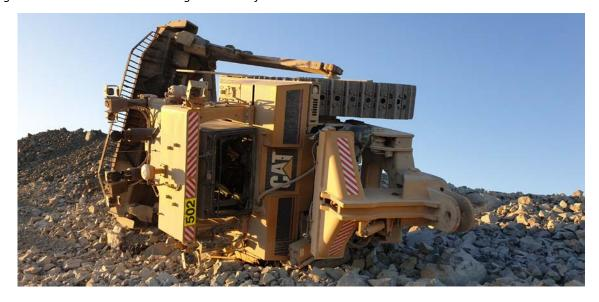
Figure 3 A dozer reversed over a light vehicle at a surface coal mine
