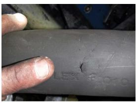
A damaged continuous miner cable arced when a worker picked it up to move it.
