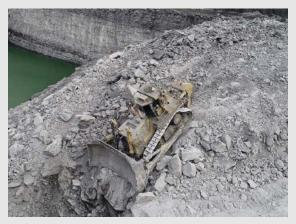
An operating dozer has pushed over onto a grade and has lost traction and become stuck.
