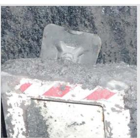
While reversing a continuous miner, the rib protection became jammed on a rib bolt causing the rib protection to deflect and strike the operator in the head.
