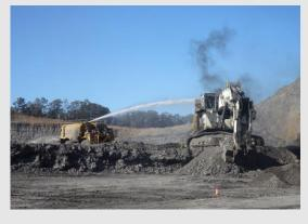
Mine operators must conduct a thorough investigation, by a competent person, to determine the root cause of any fire that occurs on mobile equipment. The investigation should include:
