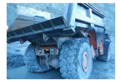
A worker was washing down a dump truck at the wash pad when the truck experienced a rupture of the rear left hand tyre involving the inside sidewall and bead.
