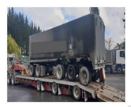
A Truck and Trailer was travelling along a state highway when the trailer wheel bearing failed and heated to extreme temperatures that resulted in a fire.
