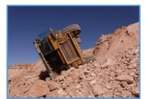
This haul truck was dumping at the edge of an over-steepened stockpile. He was wearing a seat belt and suffered only minor injuries.
