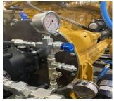
Recommended pipe configuration for pressure gauge isolation.
