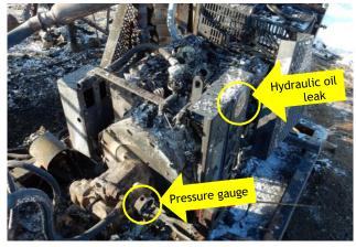
Burned engine: location of pressure gauge and oil leak
