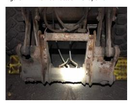
Figure 4. Gouge marks on face of workbox locking pin receptacle
