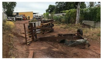
**Incident 1:** Travelling with a raised load on an uneven surface increases the risk of the forklift tipping over.
