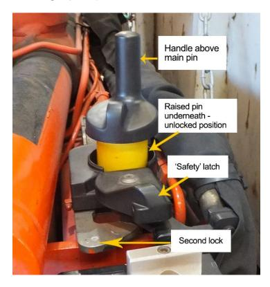
**Photograph 1**: Plastic latch un-locked and pin applicator rotated. Stabiliser ready to be extended.
