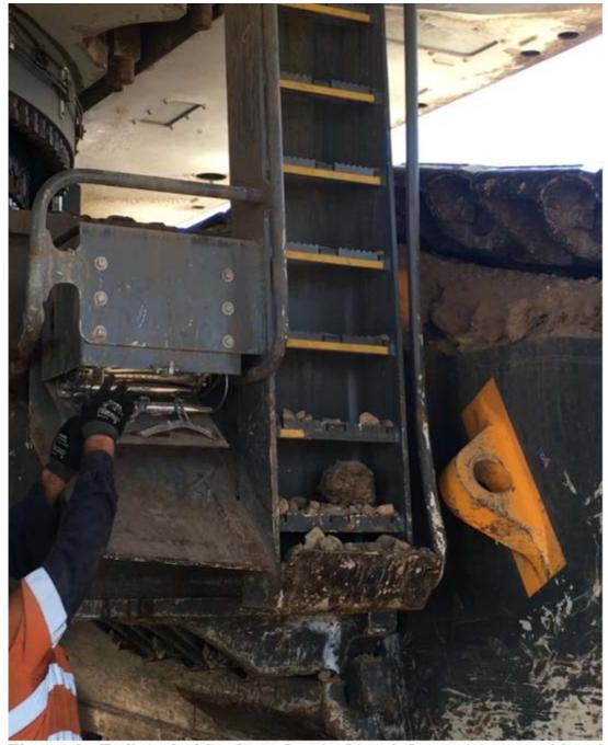
Figure 4 - Roll-up ladder from front of track frame to ground level
