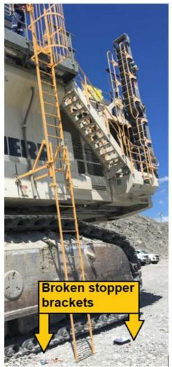
Figure 7 - Welds on both stopper brackets failed when the ladder was released
