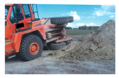
While reversing to tip his load on a stockpile, the driver of an ADT was partially blinded by sunlight and reversed up onto the edge of the stockpile. This made the loaded body unstable and it tipped onto its side.
