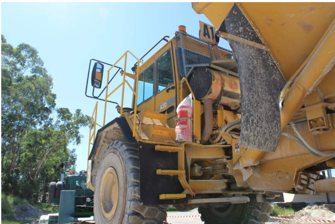
Photograph showing access handrails provided on the driver's entry door side of the Volvo A30 dump truck.
