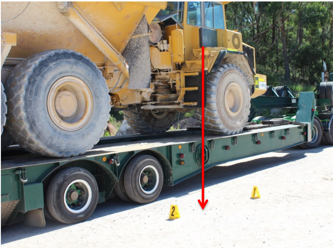
Photograph of the access ladder provided on the off-side of the Volvo A30 dump truck. The red arrow indicates the direction of the fall from the front wheel arch.
