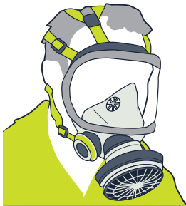
FIGURE 2: Full-face respirator (cartridge)
