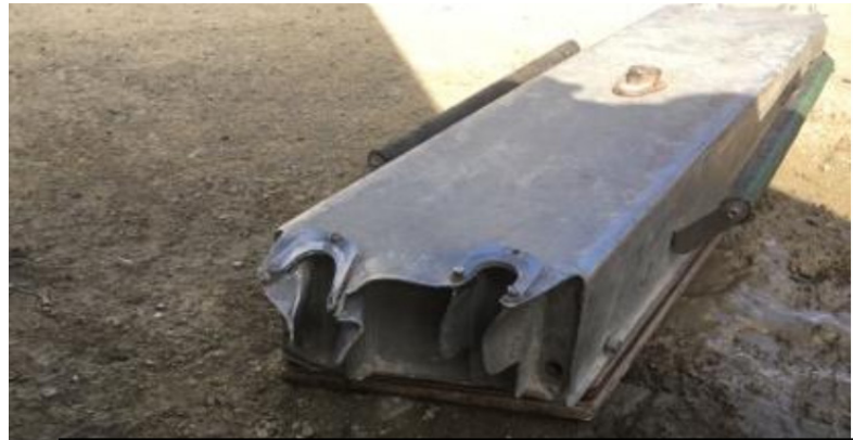
Top half of the vulcaniser where it has been bent while it catapulted off the belt
